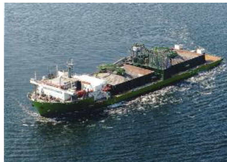
For rock placement, Tideway has the D.P. Fall Pipe Vessels 'Rollingstone' and 'Seahorse', which carry up to 18,000 t and use a DP2 navigation system
